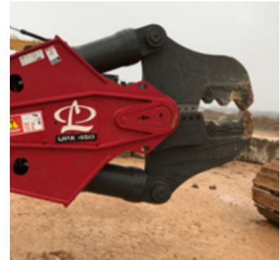
UPX 450 WITH CONCRETE CRACKING JAWS
