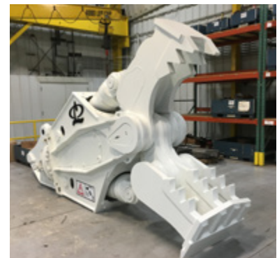
UPX 950 WITH CONCRETE PULVERIZER JAWS
