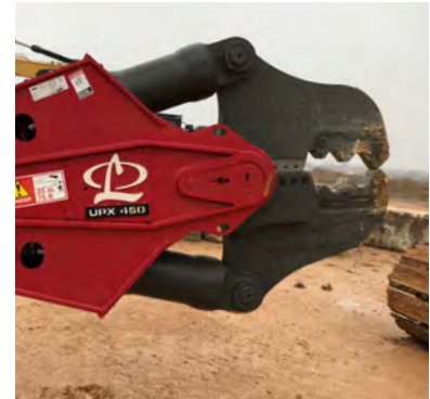
UPX 450 WITH CONCRETE CRACKING JAWS
